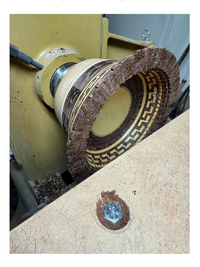
I use various negative rack scrapers to flatten the rows. It is important that the outside top edge of a flattened row is crisp.
