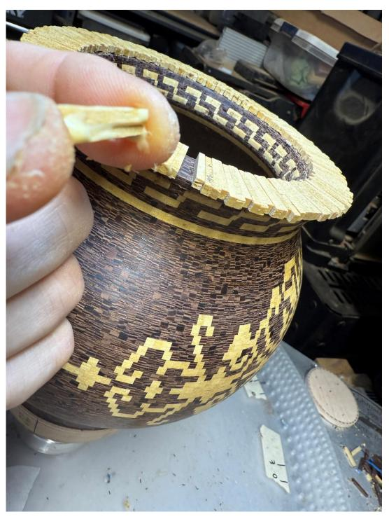
Once a segment pair is inserted, they must be pressed into position.
