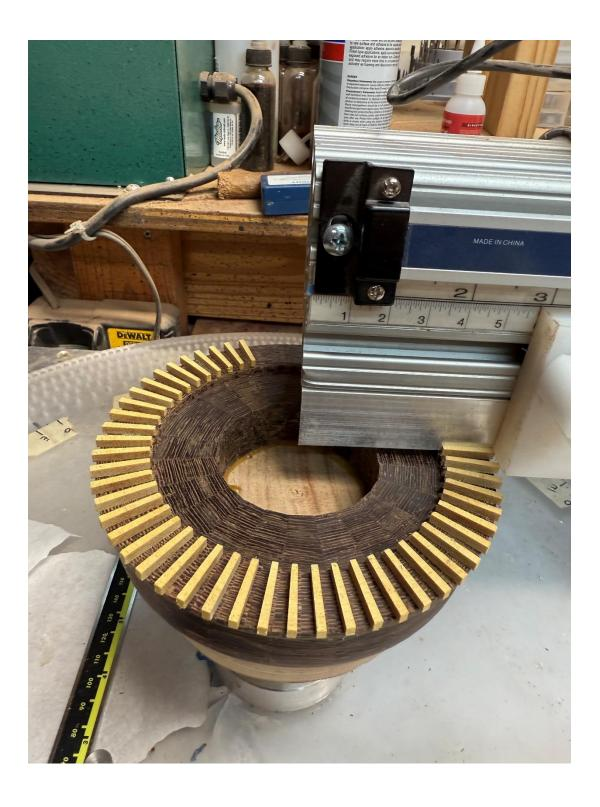
In Tom Lohman's technique every third segment is glued for a row. This leaves spaces to insert two segments between the glued segments. I use Titebond Thick and Quick glue for gluing these segments. With Titebond Thick and Quick glue the segments only need to be pressed in place for 5-6 seconds before moving to the next segment index position. I use tweezers to place and press each segment.
