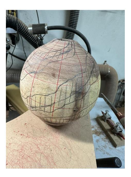
Drill holes in the area between the peel strips. These holes go halfway through the wall and are used to set the depth to be removed before piercing.
