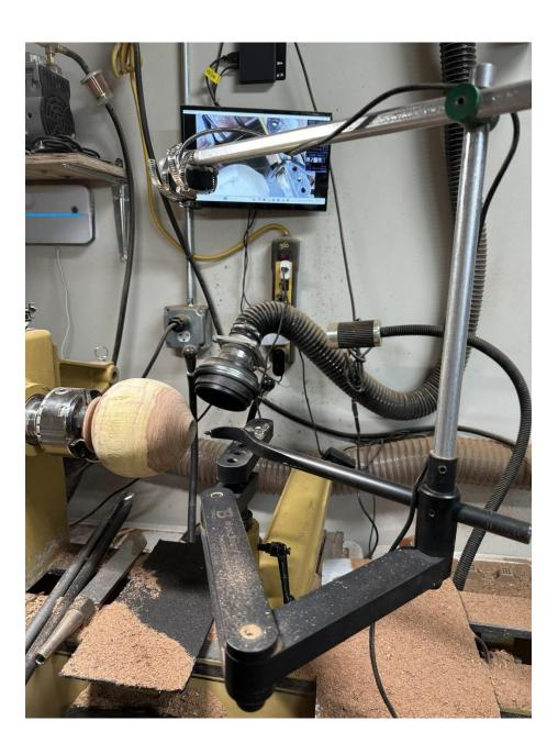
The camera-based system shows the tip of the hollowing tool inside the piece being hollowed. This facilitates hollowing to uniform wall thickness of a desired thickness.
