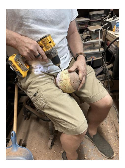
Use power carving to remove the wood between the peel strips.
