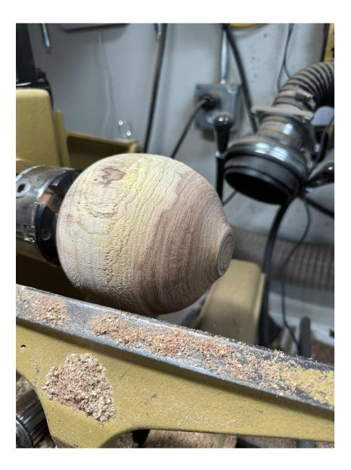
Use a 24 mm forstner bit to drill a hole to depth to be hollowed.
