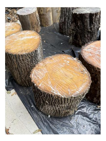
The ends of the logs are sealed using Anchor Seal. Anchor Seal is a liquid wax emulsion that dries to a layer of wax. The wax layer slows drying and minimizes cracking.
