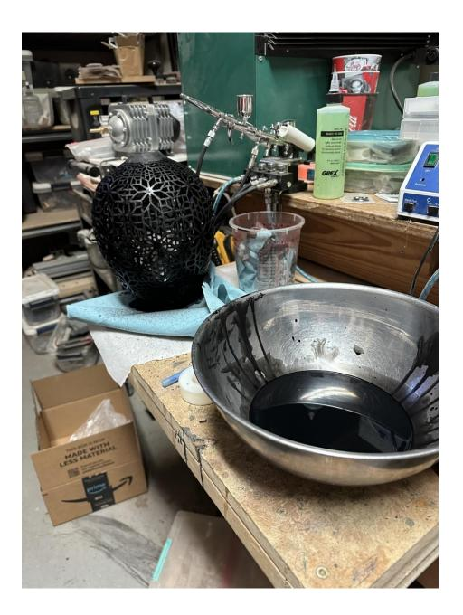
The India ink is used to blacken the inside of the piece and on the inside edges where wood has been removed. The black provides better contrast to the outside of the piece that will be sanded to reveal the undyed wood. The piece is submerged and rotated in a shallow bath of ink to insure uniform coverage.
