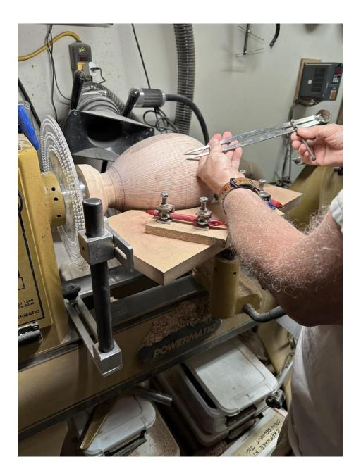
The design requires 256 longitude (top to bottom) lines. An indexing wheel with 256 indexes (clear plastic disk mounted to left of piece) and a flat platform are used to draw the 256 longitude lines. Once the longitude lines have been drawn, the flat platform is used to draw the latitude (circumference) lines around the piece. The latitude lines are positioned to create approximate grid squares. The squares are approximate because the curves of the piece distort the squares.
