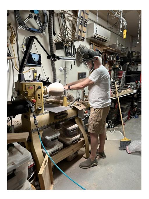
I use a camera-based hollowing system that facilitates hollowing to a uniformly thin wall thickness. I typically make the wall thickness about 4.5 mm (0.18 inch) on pieces I'm going to pierce. This thickness is thin enough to allow the drill to pierce the wood and thick enough to provide strength and contrast.
