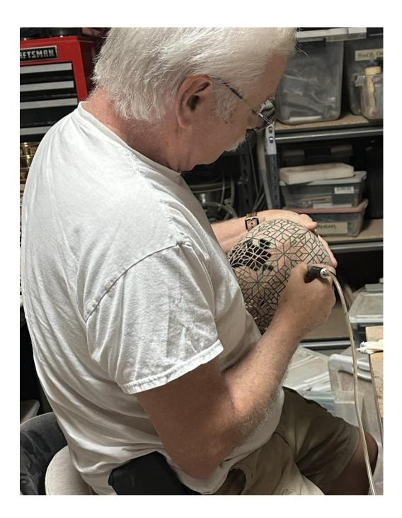
A high-speed air turbine dental drill is used to pierce the pattern on the piece. These drills are used in dental labs to shape and smooth dentures and crowns. I use an NSK Presto II drill that runs at 320,000 RPM. As a comparison, most Dremel devices max out at about 30,000 rpm. The process uses the same small carbide burs (bits) that are used in a dental lab.
